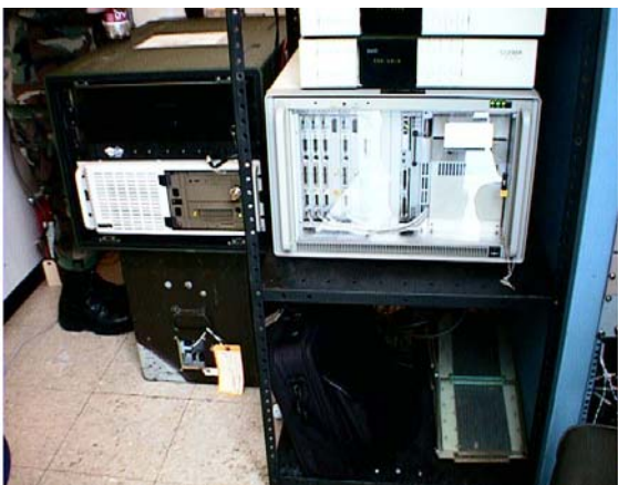
Figure 3: Solipsys MSCT Radar Simulation System on Left and Litton MTS on Right.
